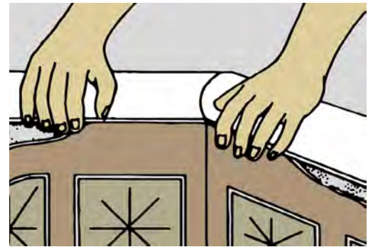
LINER BEAD INSTALLATION
